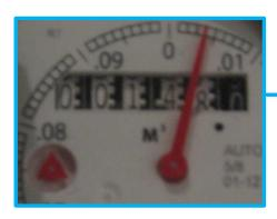
A close-up of the register to the right would indicate a reading of 00148.004 or 148.004 cubic metres.
