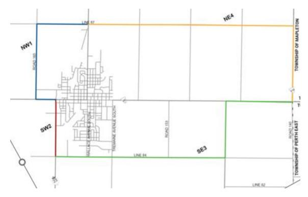
The TMP recommends implementing the proposed truck route in stages, beginning with an "east-west" route (Alternative SW2 + Alternative SE3) via Mitchell Road South/Highway 23 (between Perth Line 86 and Line 84), Line 84 (between Highway 23 and Perth Road 147), and Perth Road 147 (between Line 84 and Perth Line 86).
