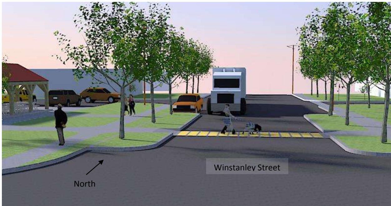
Figure 2. Trail crossing with bump-outs. Main Street looking north.
