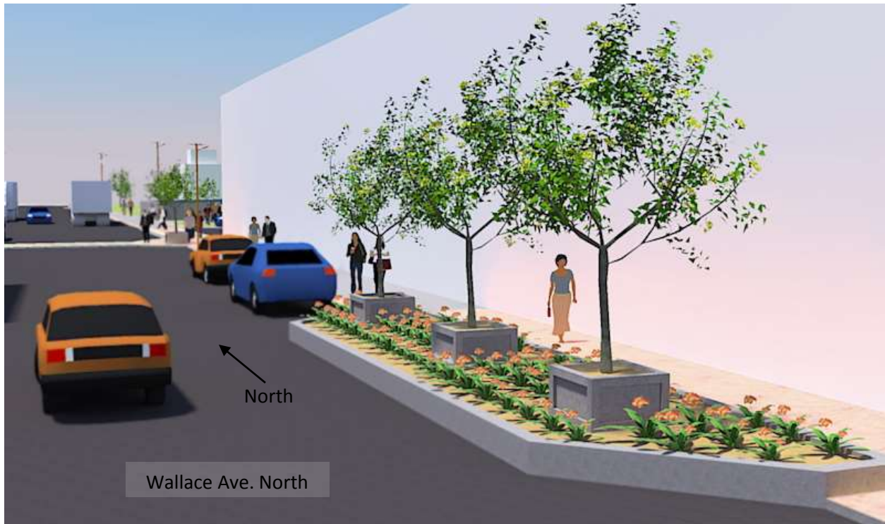
Figure 8. Raised street planter with tree boxes.
